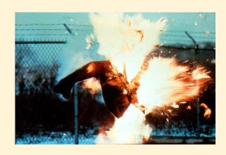
service must be designed and operated to minimize the potential hazard. This is accomplished by following the gas velocity limitations set forth in CGA Pamphlet G-4.4. By limiting the velocity, the particle impact energy is reduced, which minimizes the chance of an ignition.
