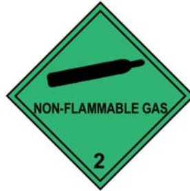
Figure 4 Nonflammable Gas Shipping Label
