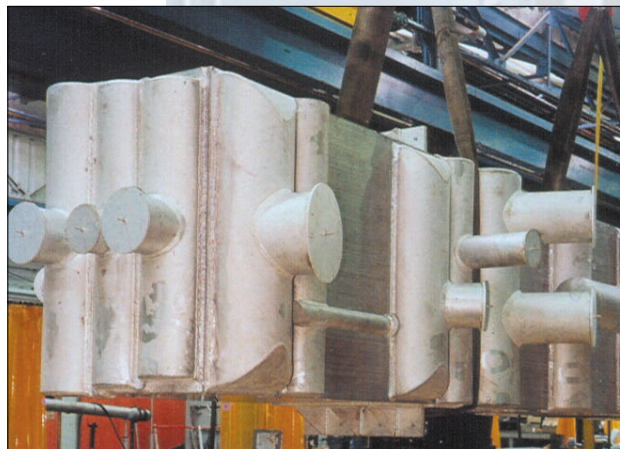
Heat exchangers from Chart Industries are designed and manufactured in accordance with Section VIII, Division I of the ASME Pressure Vessel Code, carry the "U" stamp, and are registered with the National Board of Boiler and Pressure Vessel Inspectors.
