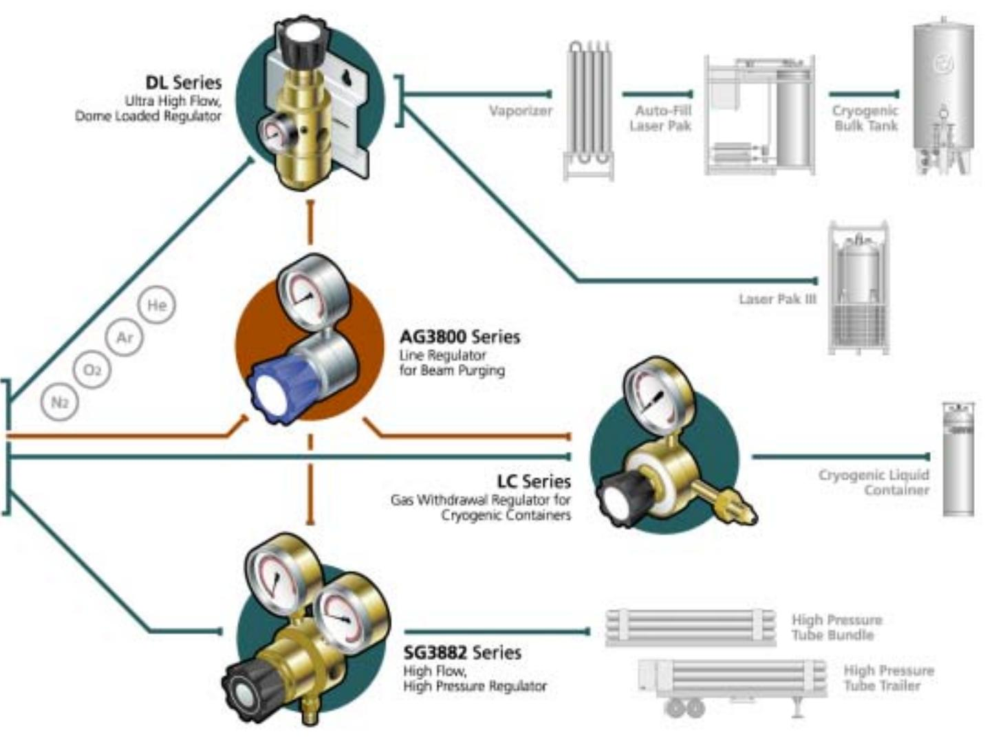
**Laser Gases** are used to generate the laser beam within the resonator. High-purity grades of carbon dioxide, nitrogen and helium are the most commonly used gases. They can be delivered to the user premixed or in component form. Maintaining a high level of purity while providing constant pressure and uninterrupted supply are the most critical requirements when selecting equipment for a lasing gas delivery system.
